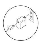
4. Plug the power block into a wall socket.5. Plug the USB connector into the power block.
