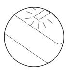
7. An orange and green light will appear when the device is initially plugged in. As a connection is being made, the light will turn orange. When the box is in use, the light will flash orange to indicate activity. When the box is not in use, there will be no light at all!
